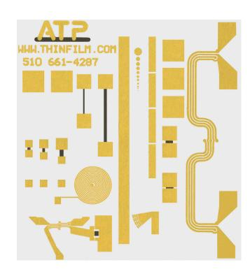
ATP offers build-to-print service for a wide range of materials and metalization schemes. ATP fabricates circuits on substrates from As-Fired Alumina to Beryllium Oxide to Fused Silica, even Silicon. Metalizations range from the standard Tan/TiW/Au to films including Nickel, Palladium, or Titanium.
